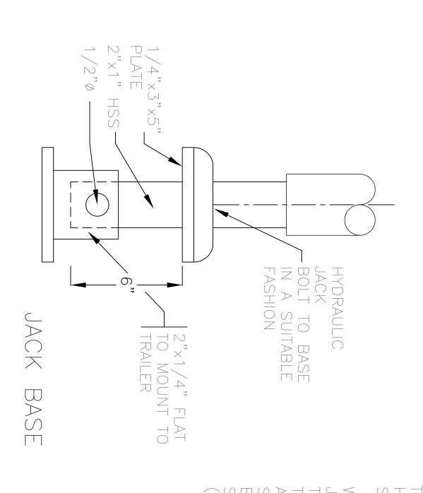
CUT LENGTH OF 2"x1" HSS SUCH THAT WHEN YOUR JACKS ARE FULLY RETRACTED THE JOISTS NEAR THE BOTTOM OF THE JUMP DO NOT QUITE CONTACT THE MAIN FRAME OF THE TRAILER.
